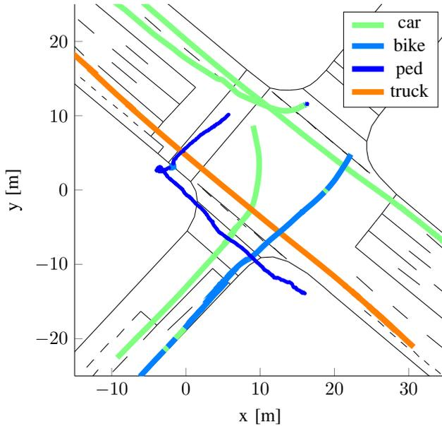
Fig. 4. Exemplary GM-CMMPHD filter tracks of one bike, pedestrian and truck respectively as well as three cars.
