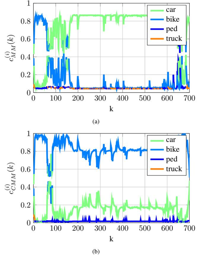
Fig. 5. Probability values of the three most probable classes of the bike track in Figure 4 crossing the intersection. (a) is the result of the filter without (MMPHD) and (b) with track features (CMMPHD).
