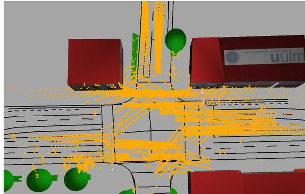
Fig. 1. Aligned range data (beam intersections with the floor) of the 14 installed laserscanners depicted in orange.
