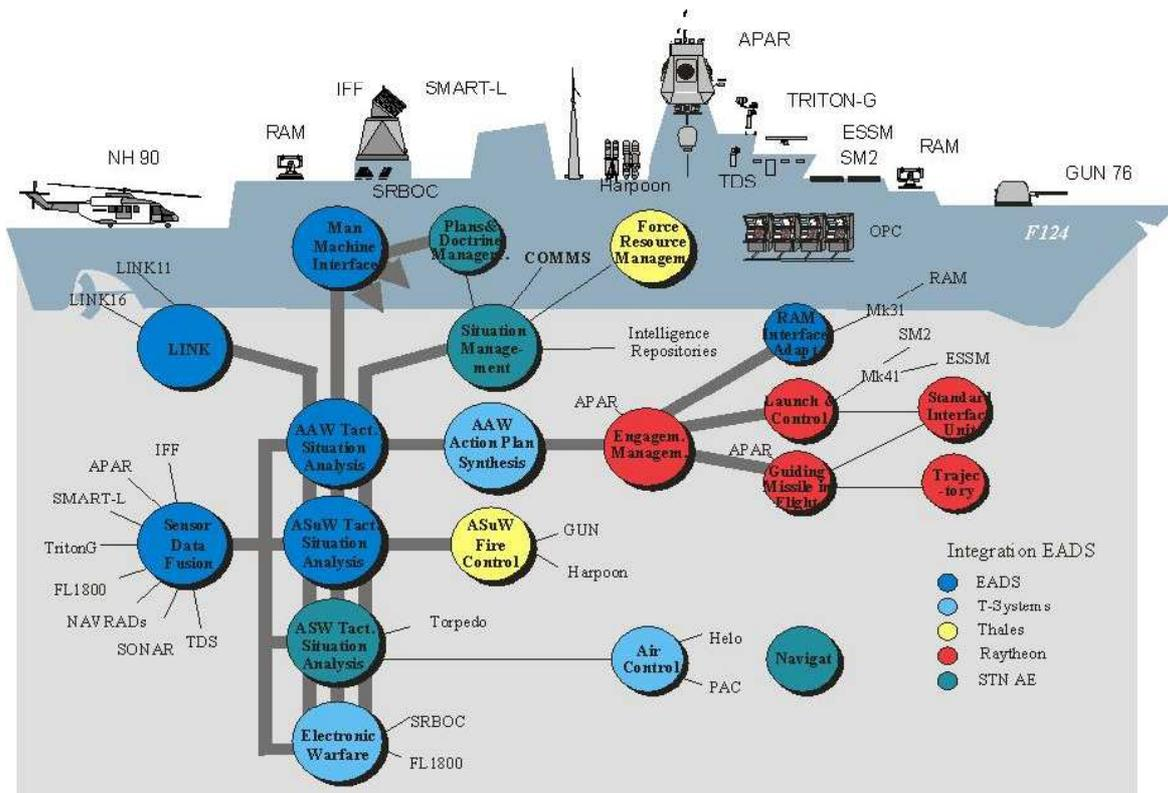
Figure 2: Frigate SACHSEN with the Combat Management System
